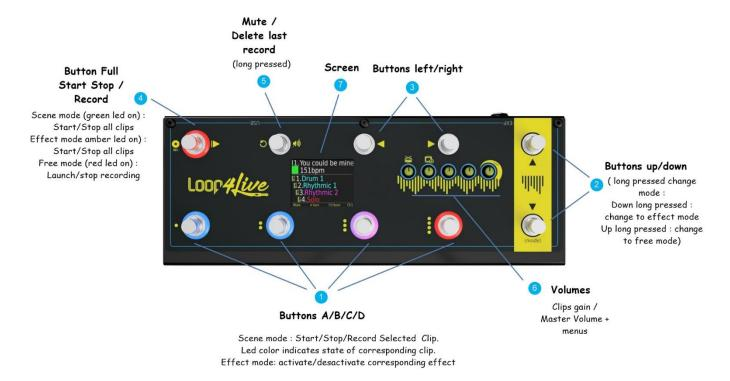
The footswitch offers 3 modes that can be selected by holding down the 2-Up/Down buttons for more than a second:
