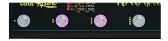
The lights around these buttons show the status of the corresponding effect (on = on, off = off).
